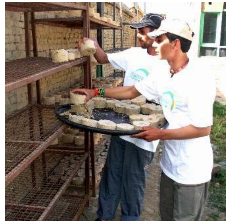
Trainees producing the fuel briquettes at the Afghans4Tomorrow Briquette Training Center, sponsored by Children's Culture Connection .
